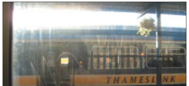
Staggering the signs fails here – a train is blocking the only visible signs
