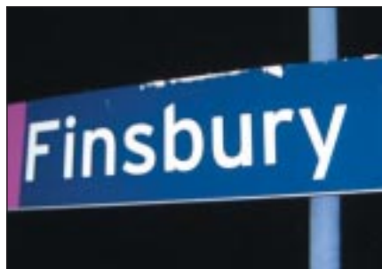
Finsbury Park (Wagn) – new applied vinyl that has already been damaged
