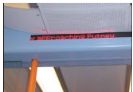
South West Trains – The LED on-board displays give station names and other information
