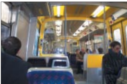
South West Trains carriage with metro seats and low seat backs (now being phased out)
