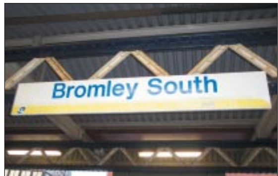
Sign size is 2100mm x 300mm 2400mm from ground to bottom of sign
