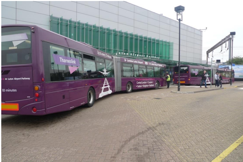
Figure 3 The bus stopping arrangement at Luton Parkway station is problematic because the bus cannot reach the kerb properly.
