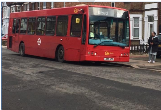
Left: Route 364 stops to pick up a passenger on its Hail and Ride section in Ilford. This road, typical of many on Hail and Ride routes, is wide enough for a fixed bus stop to be installed without affecting other road users and offers many locations with suitable kerb heights
