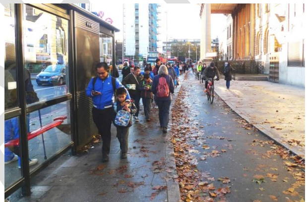
Figure 28. The cycle lane passes behind two very busy stops at Elephant and Castle.
