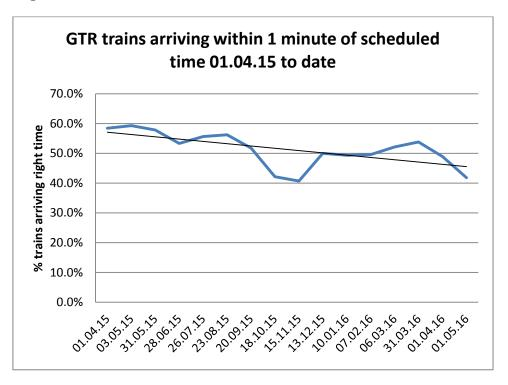
2.9 Right time arrival is a measure of the percentage of trains that arrive at their final destination either on time or early. Right time is defined as less than one minute late (and should not be confused with "on time", as defined below). The graph above shows the percentage of GTR right time arrivals in each 4-week period.
